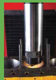
Easy & quick bore centering and machining positioning is possible with in built dial indicator
