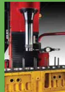
In boring spindle, you can take up the tool setting micrometer, for advantage accurate repeatable tool setting.
